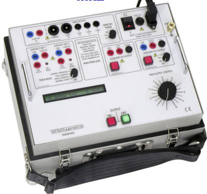
T&R Test Equipment is a market leader in the field of current injection equipment. The range includes secondary injection units with 100A output capability up to 6000A primary injection systems. All have true RMS metering, a flexible timing system, and an easy to understand user interface.
