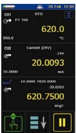
configured to show up to six reading windows and can show electrical and temperature inputs and outputs, two pressure module readings, an IDOS pressure measurement, and a USB-connected device, as well as a HART summary window or full HART communicator with active mA measurement and actual primary variable readings.
