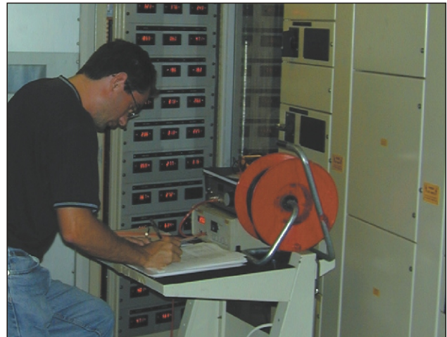
CAL95 is used to calibrate 33 Panel Mount DPM50 Sensors
